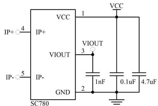
Note: 4.7uF power filter capacitors must be used to ensure performance
