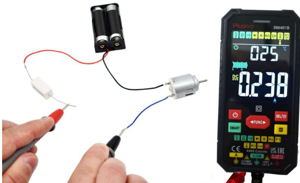
The measured current in this figure is 238 mA.
