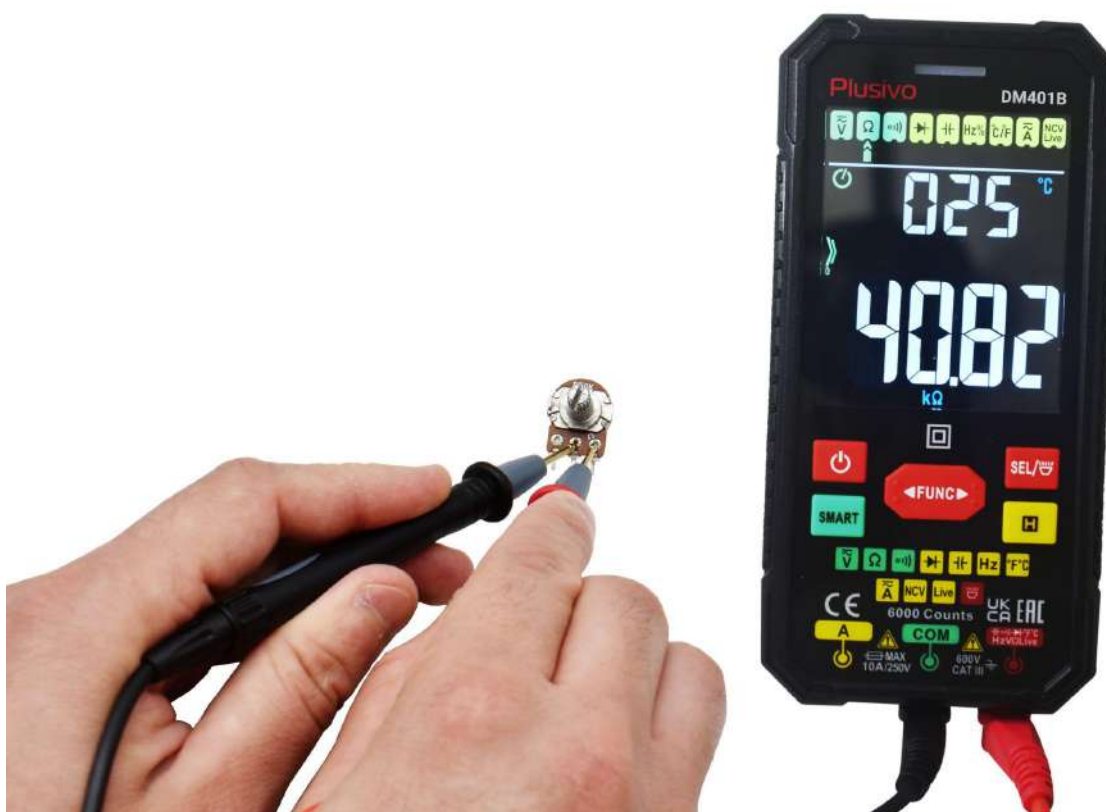
The measured resistance in this figure is 40.82 kΩ.
