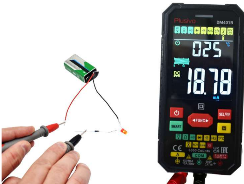
The measured current in this figure is 18.78 mA .
