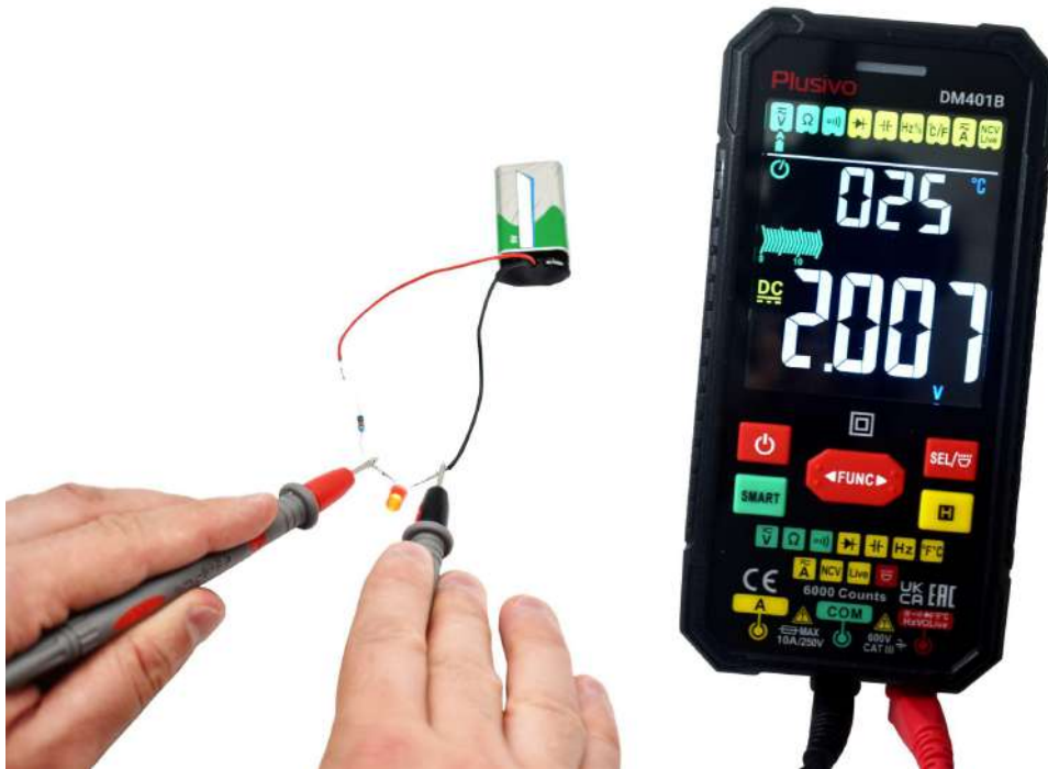
The measured voltage in this figure is 2.007 V DC
