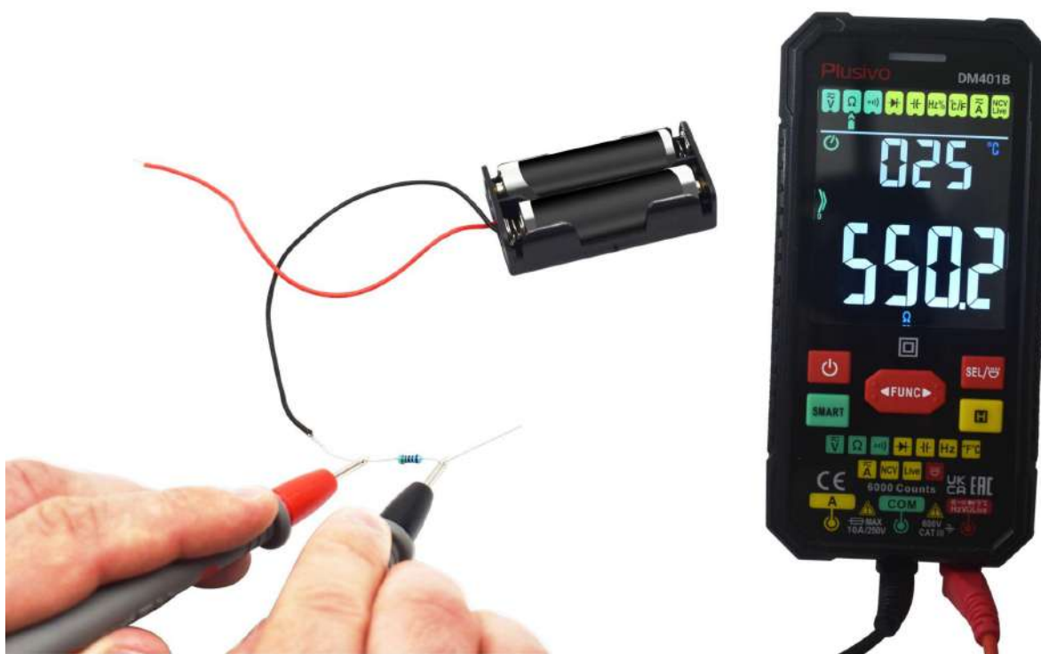
The measured resistance in this figure is 550.2 Ω
