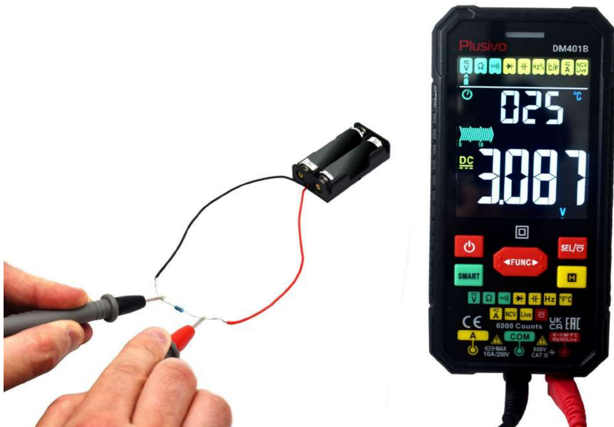
The measured voltage in this figure is 3.087 V DC.
