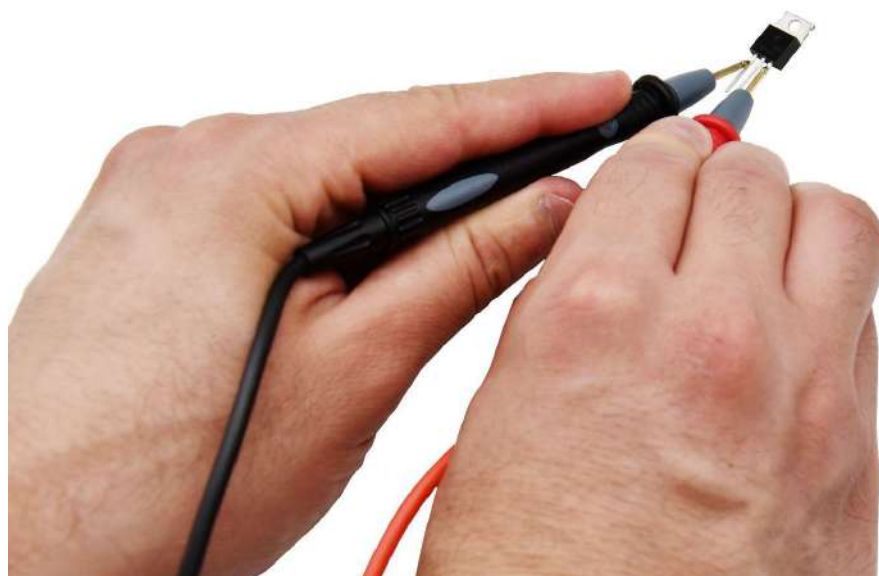
The measured forward voltage in this figure is 0.647 V.
