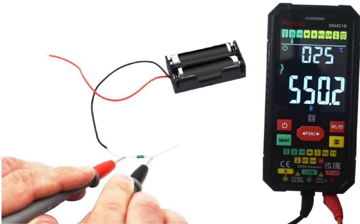
The measured resistance in this figure is 550.2 Ω .
