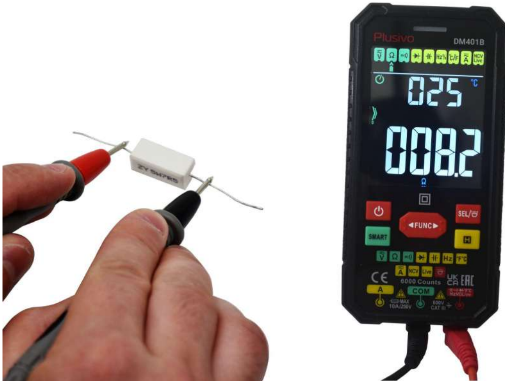
The measured resistance in this figure is 8.2 Ω.
