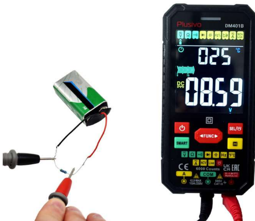
The measured voltage in this figure is 8.59 V DC.
