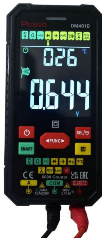
The measured forward voltage is 0.644 V.
