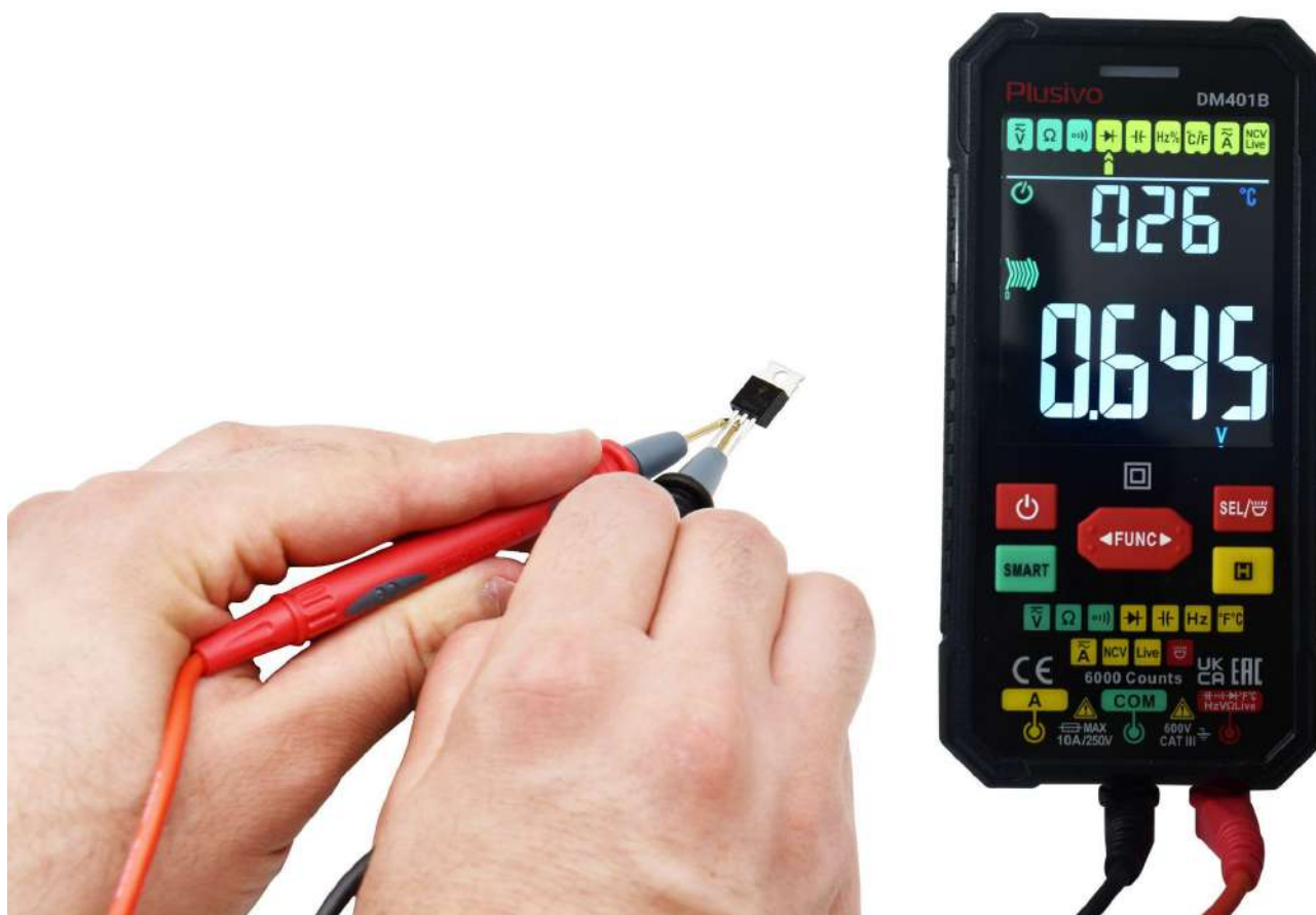
The measured forward voltage is 0.645 V.
