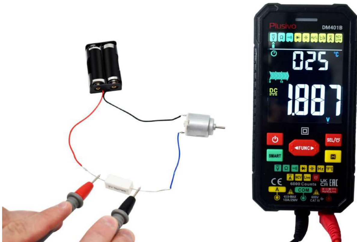
The measured voltage in this figure is 1.887 V DC.
