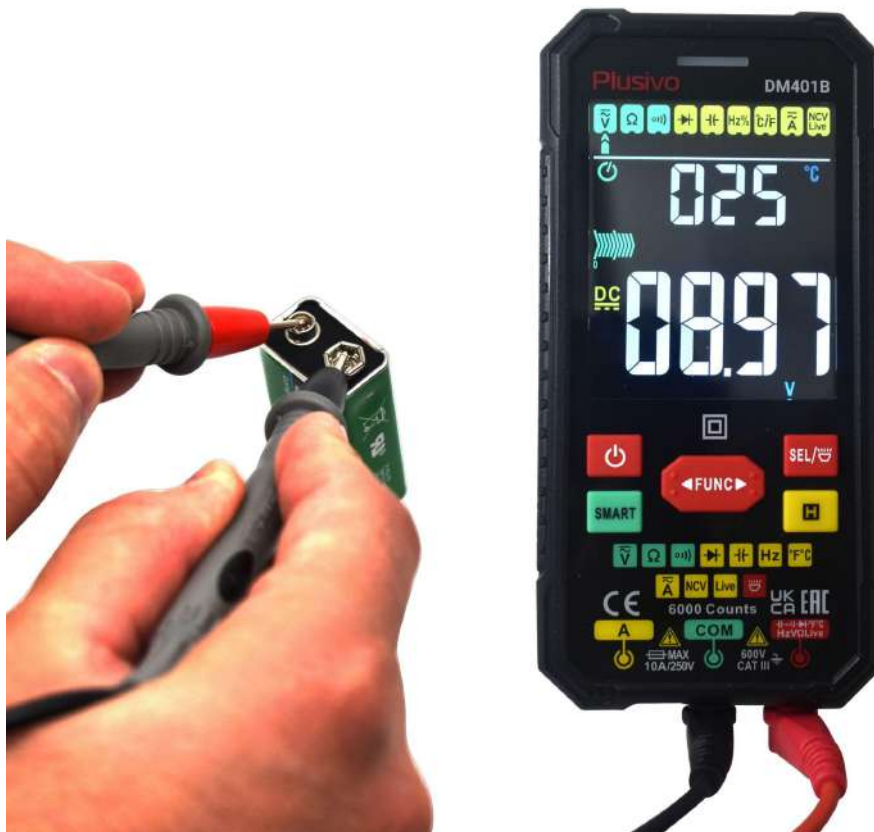
The measured voltage in this figure is 8.97 V DC.
