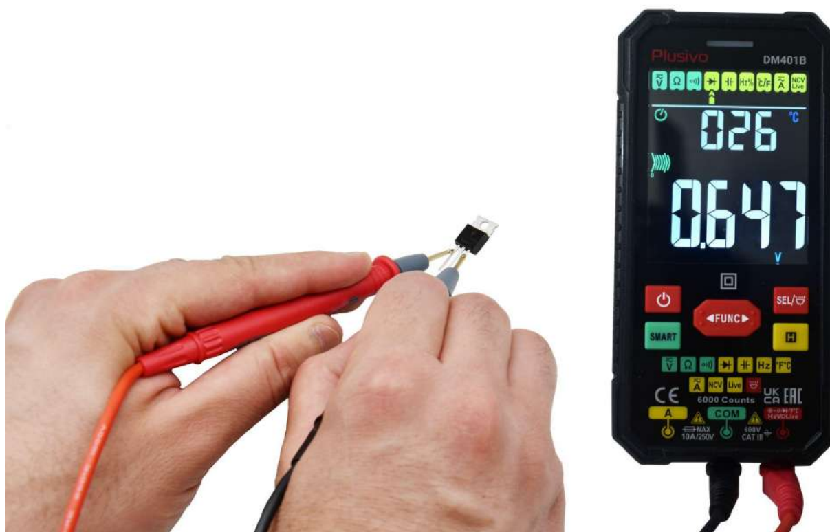
The measured forward voltage in this figure is 0.647 V.
