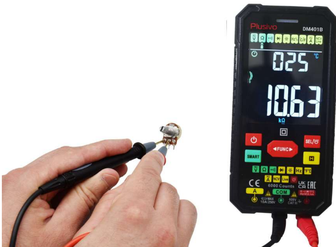
The measured resistance in this figure is 10.63 kΩ.
