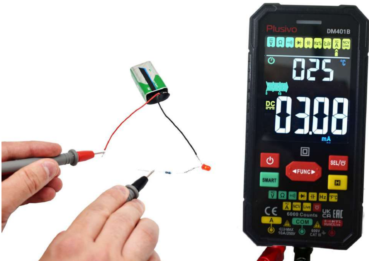
The measured current in this figure is 3.08 mA.
