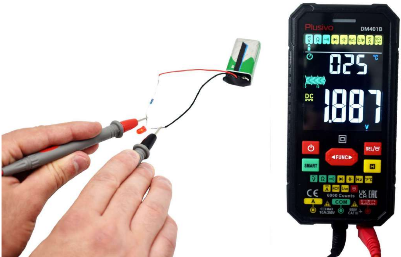
The measured voltage in this figure is 1.887 V DC
