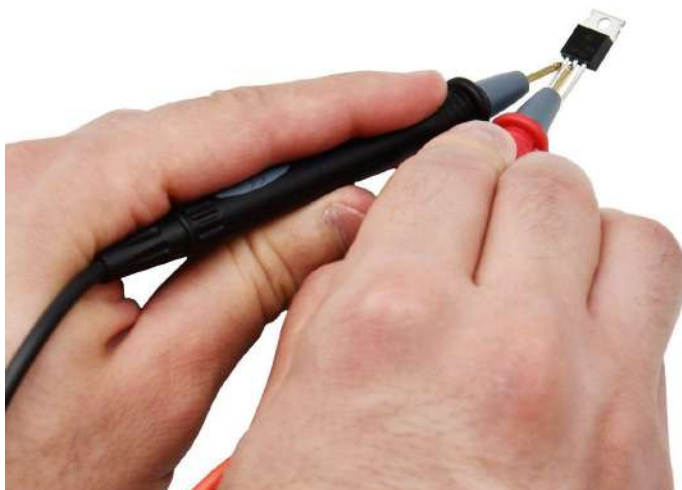
The measured forward voltage is 0.644 V.
